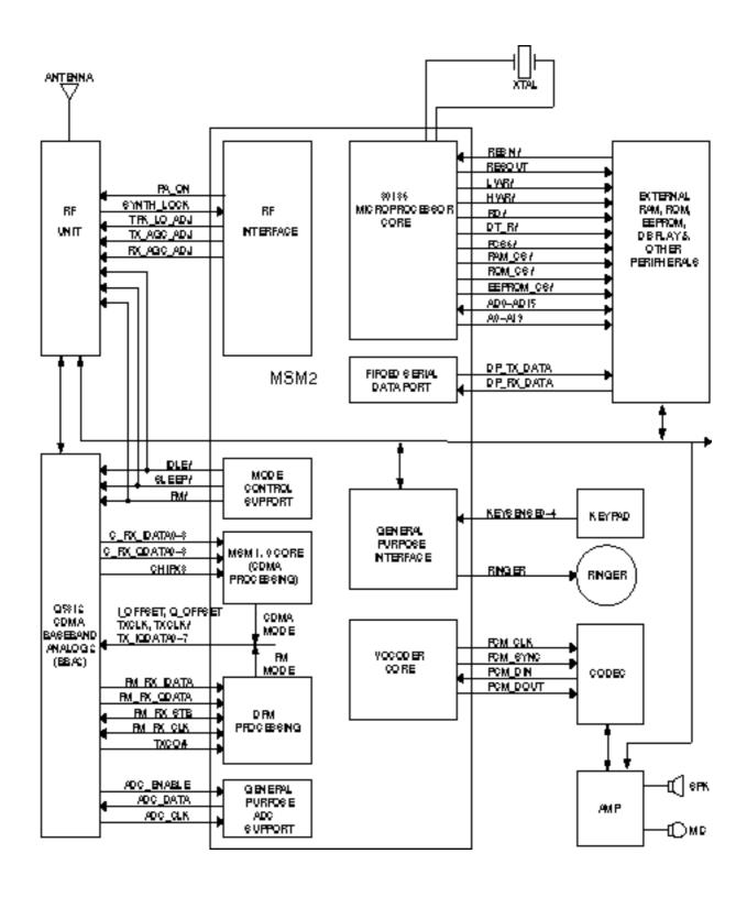
Figure 6-1 Baseband Block Diagram
